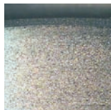
DiamondFaces®: Sliding faces in good condition after 11500 h, no leakage
