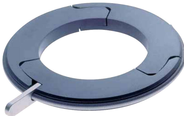
Multi-part sealing ring, with gas-tight joints having overlapping mortise
